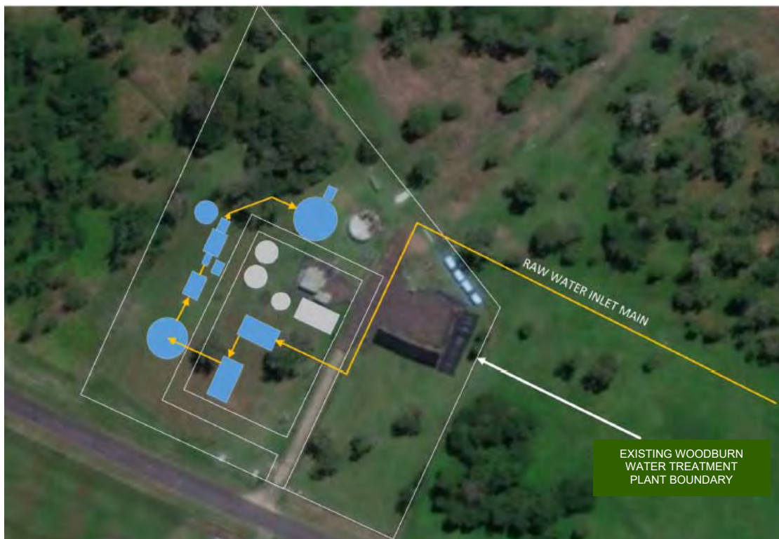
Figure 12: Woodburn groundwater WTP inlet and layout
