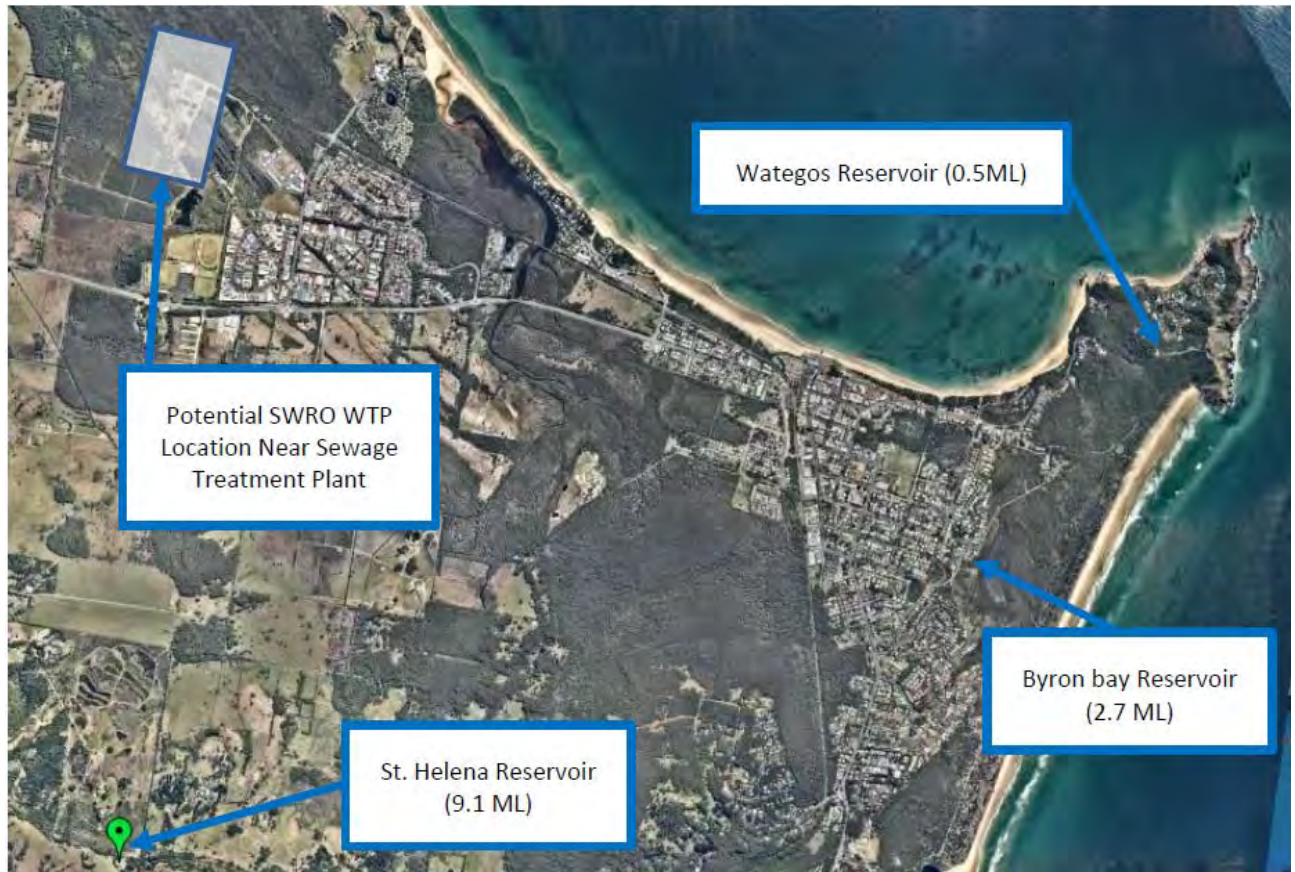
Figure 14: Proposed desalination plant location in Byron Bay
